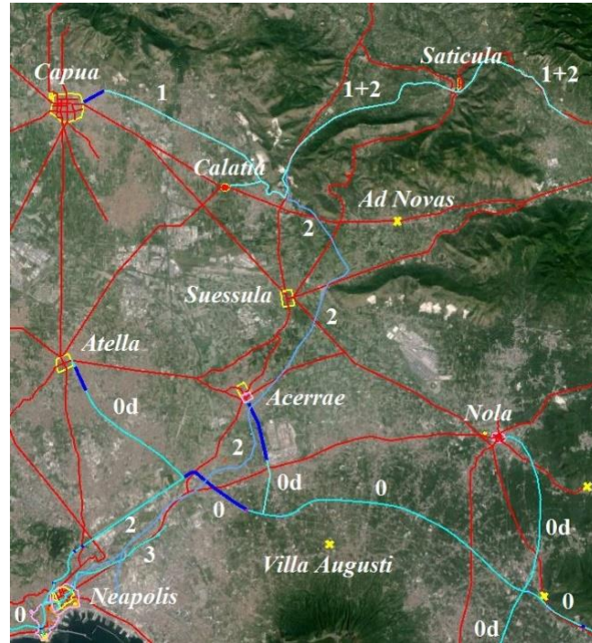
Fig. 6 - Overall view of the route of the Carmignano aqueduct. It is also drawn the course of Aqua Julia aqueduct which should be identical, or nearly so, to that of Carmignano aqueduct for “circa 8 miglia” (about 8 miles). Moreover, the map shows also the civitates served by the oldest aqueduct, the road network allegedly existing in Roman times, and the course of the Augustan aqueduct of the Serino. 0: Augustan aqueduct of the Serino; 0d: branches of this aqueduct; 1: Aqua Julia aqueduct; 2: Carmignano aqueduct; 3: Bolla aqueduct; 1+2: parts of 1 and 2 in common.
